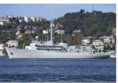
• **R/V Cesme**: Length 87.00m; Freeboard to Work Deck (m) 3.0; Draft (m) 4.6; Gross Tons 2900.0; Fuel Capacity (m³) 346.0; Area Wetlab (m²) 30.0; Free Deck Area (m²) 150.0; Space Cont Labs Supported (m²) 100; Range (n mi) 8000.0; Speed Cruise (kt) 12.0; Speed Max (kt) 15.0; Endurance (days) 50.0;
