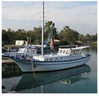
• R/V Lamas (wooden hull): built in 1981; Length: 16 m; Tonage: 28 Gross; Draft: 1.60 m; Speed: 11.5 knot; Accommodation – crew 3 and scientists 4. The Trawler is used mostly in biological and fisheries surveys but is also capable of oceanographic investigations. Equipment: JRC Fisheries echosounder (Fish finder) (50 & 200 kHz); Garmen GPS; Oceanographic winch; Sentinel Workhorse ADCP (300kHz); Wireless communication device.
