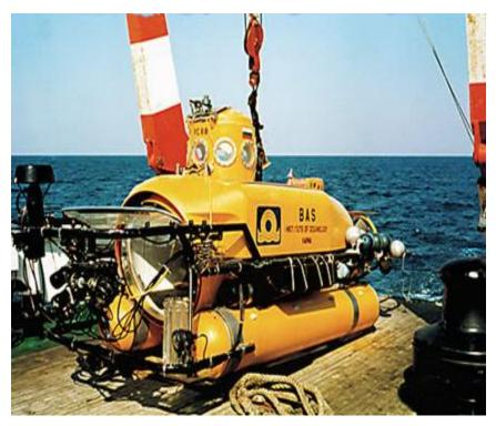
• Research Submersible PC-8 - The research submersible PC -8 has been operated since 1987. Main characteristics: Operating depth - 250m, Deadweight - 5t, Length - 6,5m, Crew - 2+1, Range of underwater cruise - 5 n miles, Endurance underwater - 5 hours, Scientific equipment - photocamera, video-camera, manipulator, sampling devices
