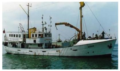
R/V Avar: Built in 1951; Length 31.27 m; Draft 3,20m; Tonnage 173,68 gross tons; Length 31.27; Draft (m) 2.76; Gross Tons 178.0; Capacity Dry Cargo Area (m³) 3.0; Fuel Capacity (m³) 30.0; Area Wetlab (m²) 8.0; Area Drylab (m²) 10.0; Free Deck Area (m²) 55.0; Range (n mi) 5000.0; Speed Cruise (kt) 9.0; Speed Max (kt) 11.0; Endurance (days) 30.0; Accommodation - Officers 2, Crew 11, Scientists 15; Air
