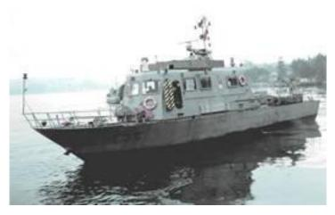
• **R/V Mesaha 2**: built in 1994; Length/Breadth: 21.28 mt/5.07 mt; Displacement: 47 ton Draft: 1.33 mt; Maximum Speed: 10 KTS; Endurance:400 mil; Main Engine 2 x 1000 HP; Accommodation: Crew 10 and Scientists 5.
